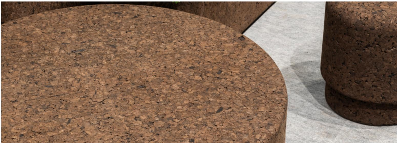
Expanded cork is itself, in a way, a by-product of the traditional cork industry. Expanded cork is made from the bark of the cork tree that is of too poor a quality to be used for making natural wine corks. It is manufactured from the cork bark of the upper branches of the cork oak tree. This bark is
